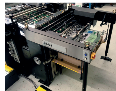
The sheet feeder is open and easy accessible for the operator to load and / or correct the sheet pile.
