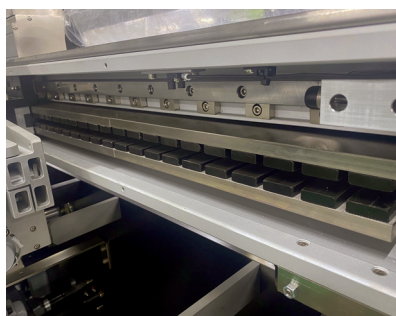
Linear electro-magnetic drive for the screen carrier R.
