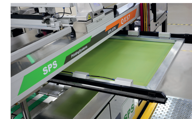
Simply slide the screen into the machine from the operator side.
