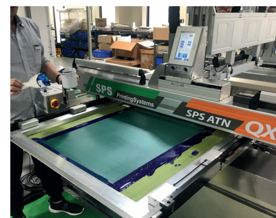
Inspection and / or cleaning top and bottom side of the screen; holding perfect registration when pushed back into the machine.
