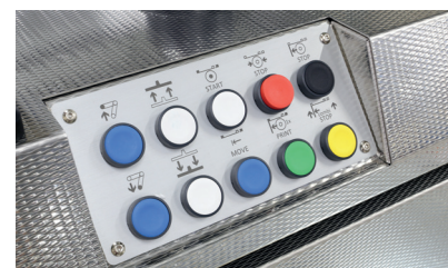
Extra operator panel with hard buttons for the most used machine commands, located at the sheet exit side.
