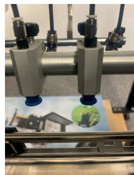
Individual spring-loaded suction elements for optimized sheet separation.
