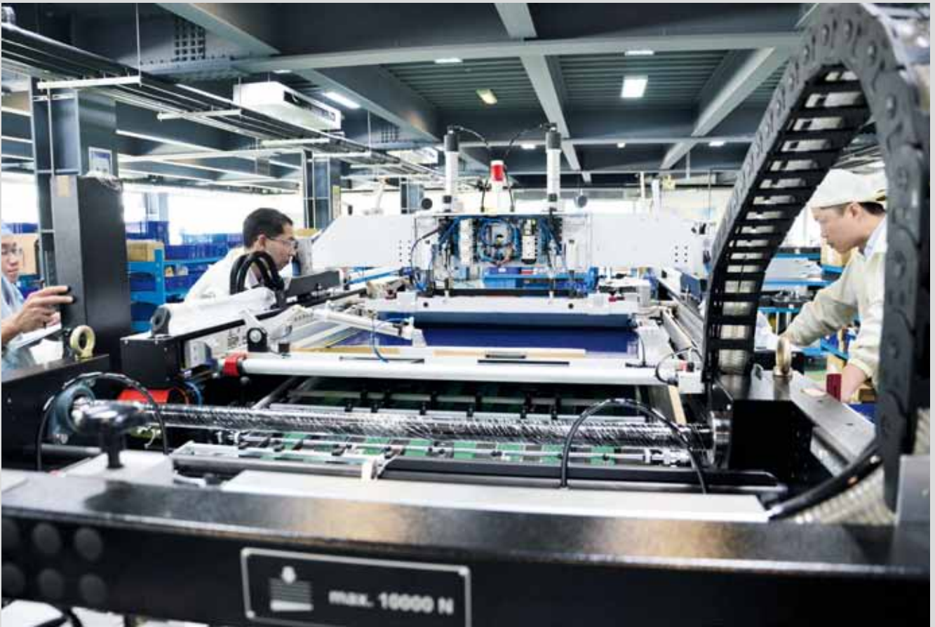
A cylinder screen printing machine, which is manufactured for the German partner SPS
