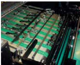
Anti-static upgrade for industrial applications on film substrates: fan blowers and underside electrode.
