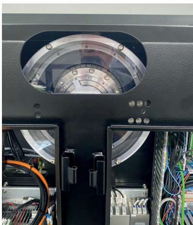
Servo-motor main drive direct connected to the cylinder.
