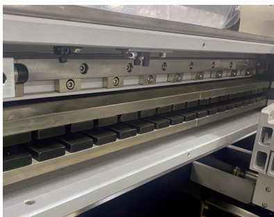
Linear electro-magnetic drive for the screen carrier L.
