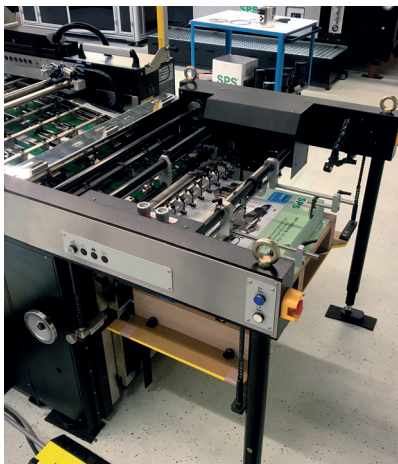
Single sheet, front pick-up feeder for scratch-free separation from the pile.
