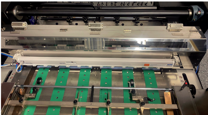
(Optional) both top and bottom sheet cleaning system, blue pick-up roller transferring dust particles to the adhesion roller; (optional) anti-statics.
