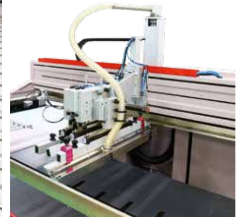
Stable speed printing head carriage + auto ink dispenser (option)
