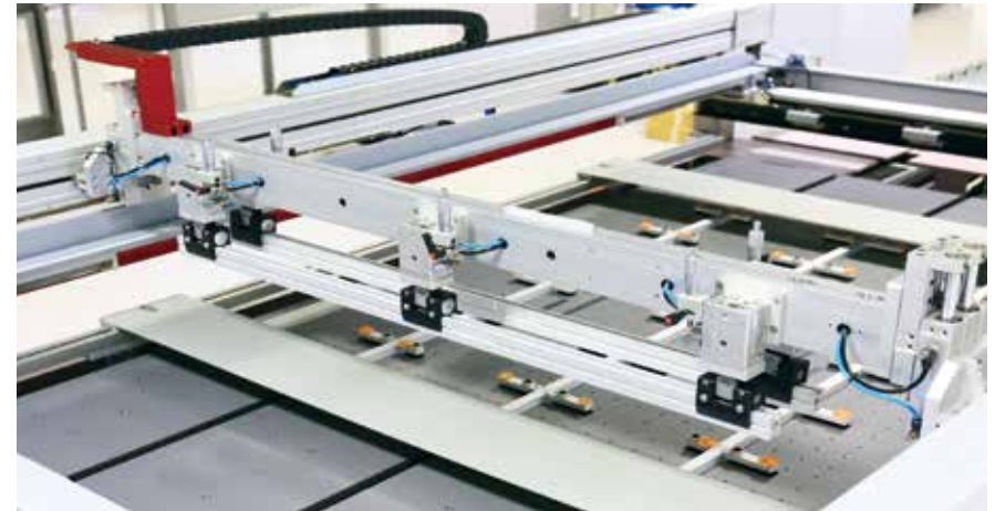
Printing head carriage and nesting bar structure
