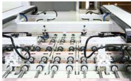
Correcting structure above feeding
