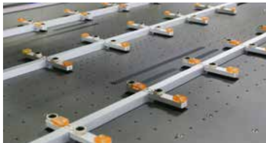
Double vacuum carrier shuttle transfer
