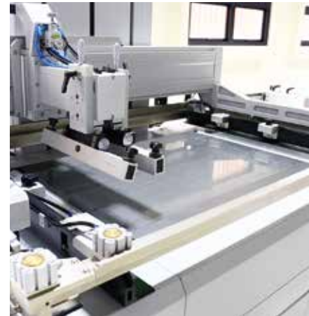
Printing head carriage and screen frame structure
