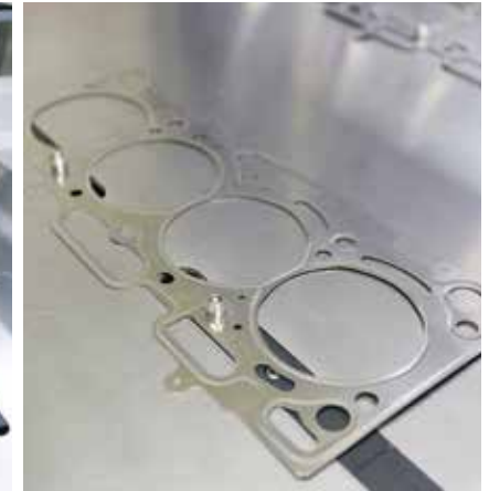
Equipped with registration pins on table
